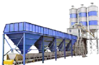
Concrete Batching Scale
